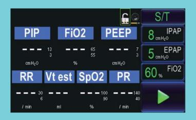
The S/T Mode of the OmniOx ventilator delivers pressure support with PEEP. The unit triggers Inspiratory Positive Airway Pressure (IPAP) in response to spontaneous inspiratory effort and cycles to Expiratory Positive Airway Pressure (EPAP) during exhalation.
